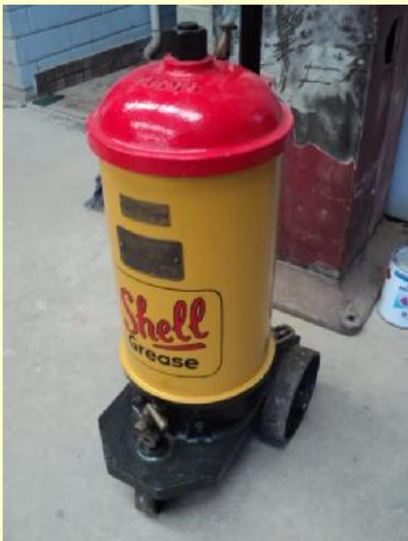
Steve Murphy recently purchased this Shell logoed greaser fro Tasmania. It's labelled as being the JASCO Garage Lubricator Model A Lubricator, made in Melbourne.
